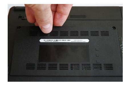
8. Snap the backplate back on, and screw in the two retention screws.
