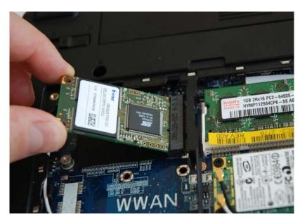
5. The stock SSD will pop up on its own after the screws are removed. Pull out the stock SSD.
