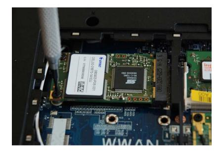
4. Locate the SSD and carefully remove the two retention screws. Be careful not to drop the screws into the computer.
