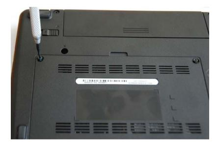
2. Locate the removable backplate on the bottom of the Mini 9. Unscrew the two retention screws.
