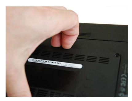
3. Gently pry open the backplate with your fingers. Even after the screws are removed the backplate is still snapped in place.
