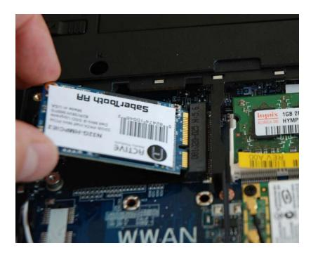
6. Slide the SaberTooth SSD into the Mini PCIe slot, making sure the key in the SSD lines up with the key in the connector.
